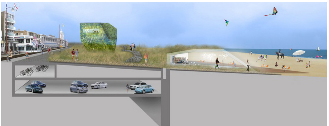
An example of parking under the foreshore also acting as a dike, protecting the shoreline. Katwijk Aan Zee, The Netherlands
